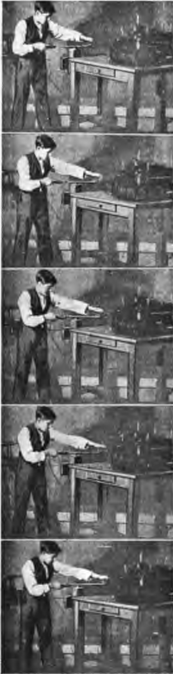
FIG. 66. Apprentice (Fitter) filing Metal. To the left, the Correct Attitude; to the right, the Incorrect. (The Sequence of the Pictures is from Top to Bottom.)
